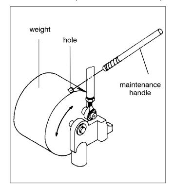
Figure 1-13. Removable maintenance handle on 4000 amp. F–design transfer switch.
